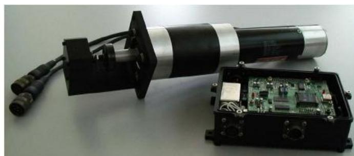
Figure 4. Servo Actuator
