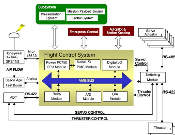
Figure 1. Autonomous Flight Control System
