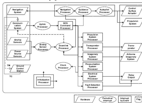
Figure 5. Software Structure of Flight control
